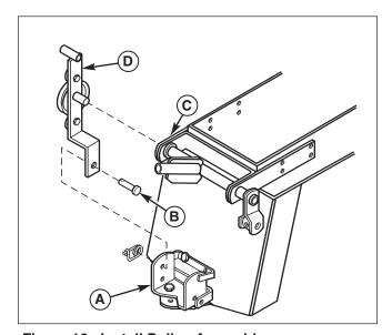
Figure 16. Install Pulley Assembly
